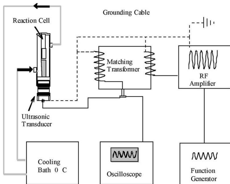
**Figure 2. The Variable Frequency Sonicator.**
