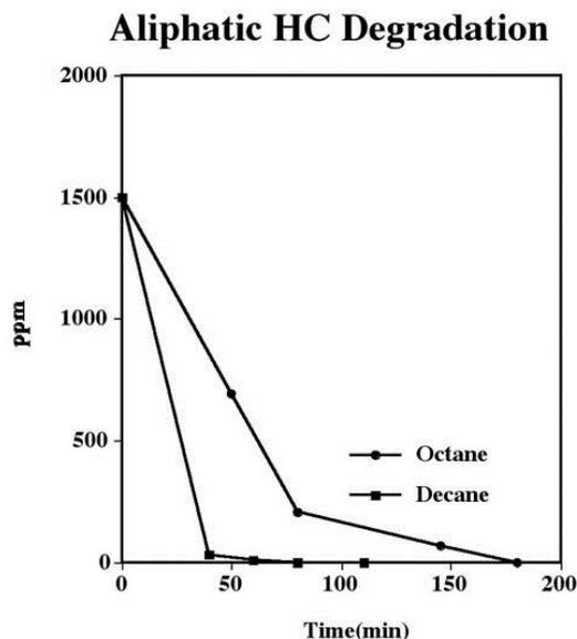
**Figure 1. The sonolytic degradation of octane and decane in water.**
